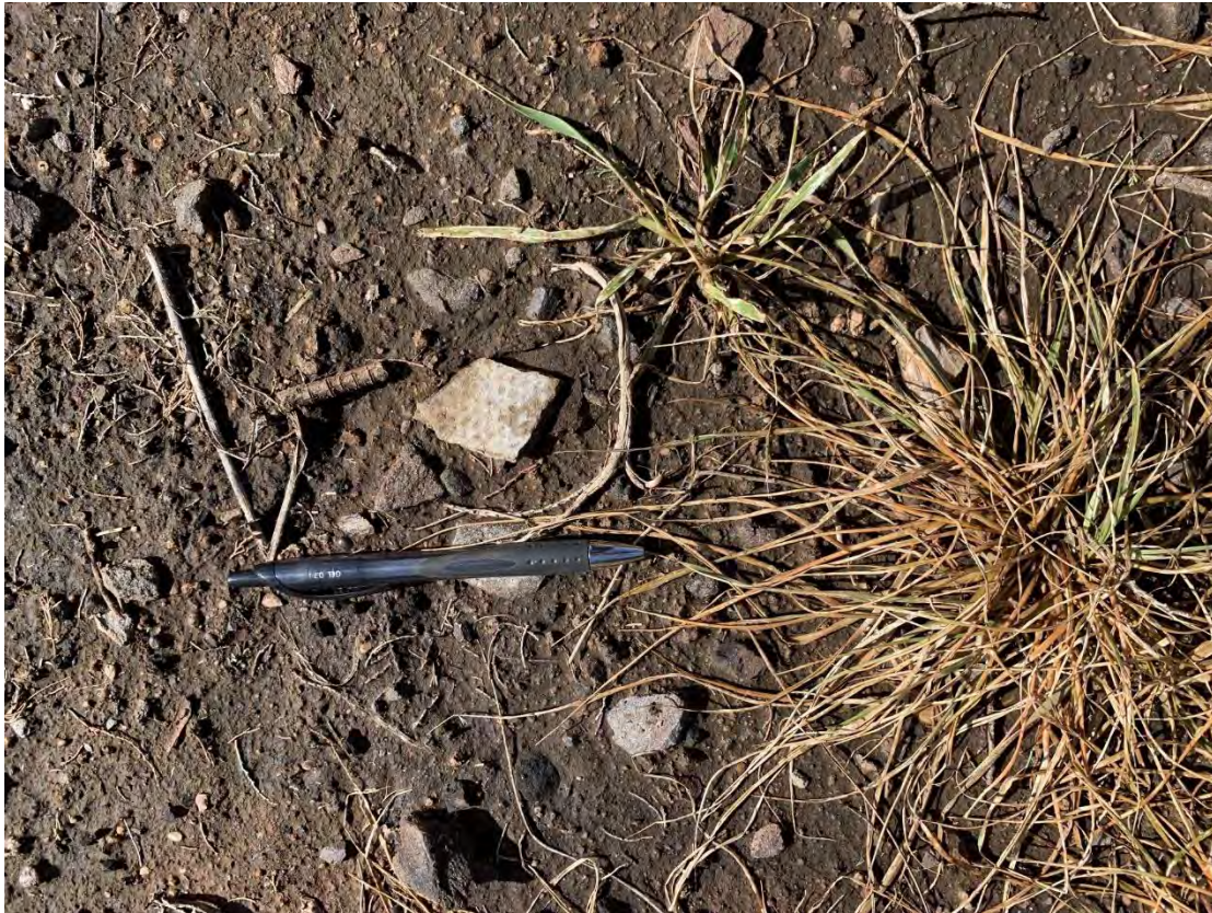
Photograph 11: An ACM fragment on the demolished house and garage site.
